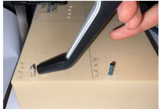
Fig. 5 Representative image of the 3p S implant stability quotient (ISQ) measurements in the mesial and distal orientations, after insertion into a 40 PCF polyurethane bone block
